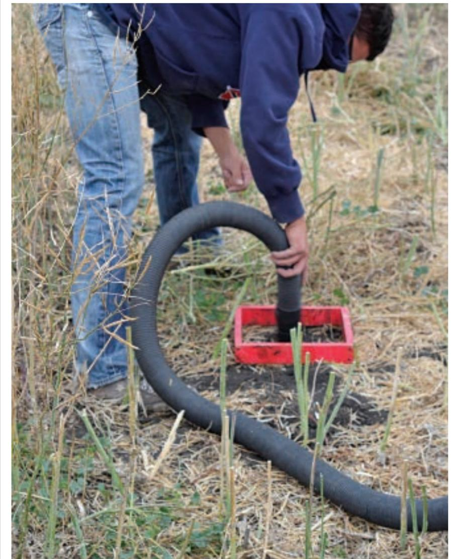
To measure harvest losses, all soil and crop debris, including dropped seeds, are vacuumed. Seed is then separated from the sample, and weighed.
