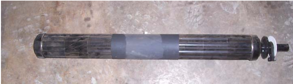
Figure 7. Long External Flutes Extra Fine Metering Roller.
